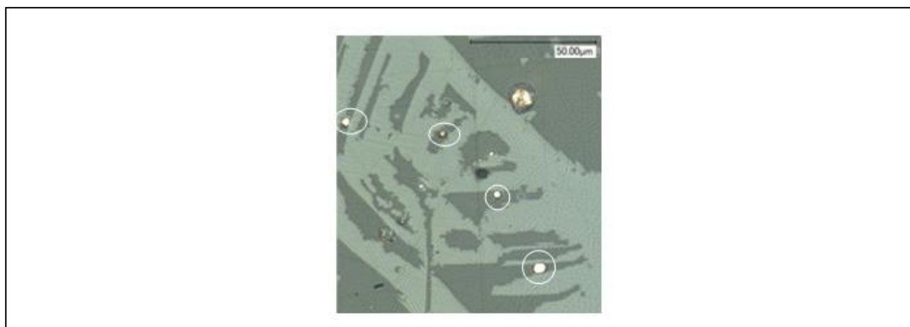
Figure 5: Experimentally obtained micrographs of Cu droplets within a cavity inside a solid particle indicated by white circles [21]
